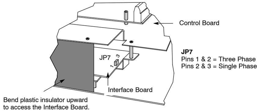
**Figure 3-8 Size C2 Single Phase 230/460VAC Power Connections**
