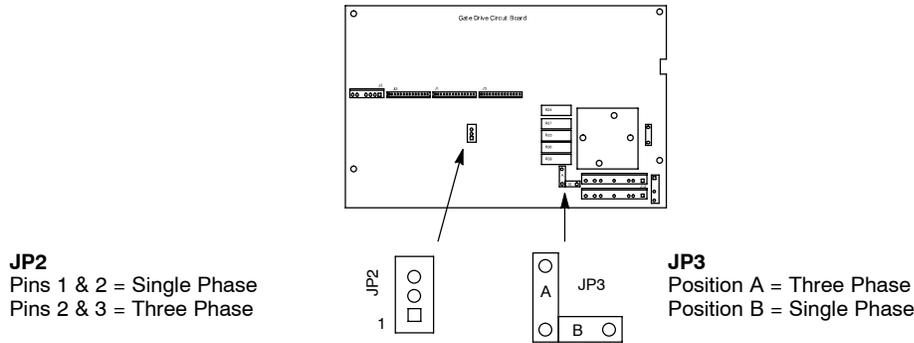
**Figure 3-10 Size D Single Phase 230/460VAC Power Connections**
