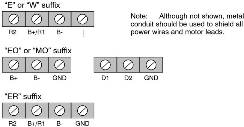
**Figure 3-18 Wiring for RGA Assembly**
