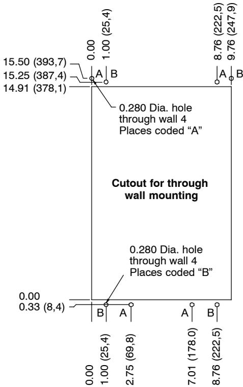
Note: Throughwall mounting provides NEMA 4 protection. For clarity, cover and inside components not shown.
