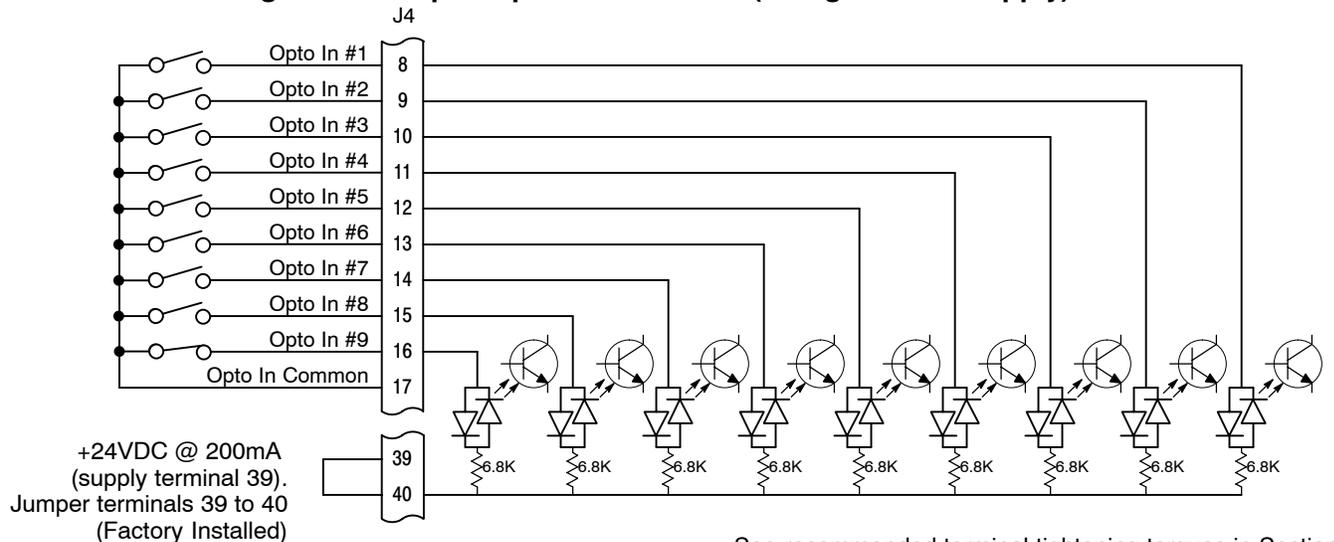
**Figure 3-35 Opto-Input Connections (Using External Supply)**
