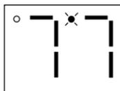
In the example above, Parameter 54 - MOTOR LOAD is being viewed. The “77” in the example indicates that the load on the motor is 77% of the output current rating of the drive.
