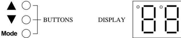
To enter the PROGRAM mode to access the parameters, press the **Mode** button. This will activate the PASSWORD prompt (if the password has not been disabled). The display will read "00" and the upper right-hand decimal point will be blinking, as shown below:
