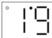
Once the desired parameter number is found, press the **Mode** button to display the present parameter setting. The upper right-hand decimal point will begin blinking, indicating that the present parameter setting is being displayed, and that it can be changed by using the ▲ and ▼ buttons.
