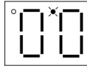
Use the **▲** and **▼** buttons to scroll to the password value (the factory default password is "25") and press the **Mode** button. Once the correct password value is entered, the display will read "01", which indicates that the PROGRAM mode has been accessed at the beginning of the parameter menu (01 is the first parameter), and the upper right decimal point will turn on solid. This is shown below:
