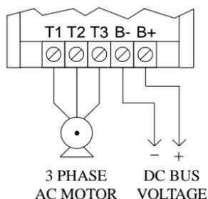
3 PHASE AC MOTOR      DC BUS VOLTAGE
