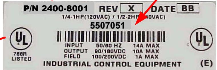
Always record the drive **Model Number**, **Part Number** and **Serial Number** for future warranty situations and spare parts. A good location to record these is on the [Start-up Guide Worksheet](#) on page #41.
