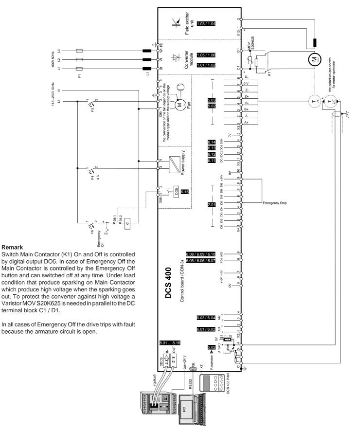
Fig. 5.3/5: Connection example for Emergeny Stop - DC breaker with drive coasting
