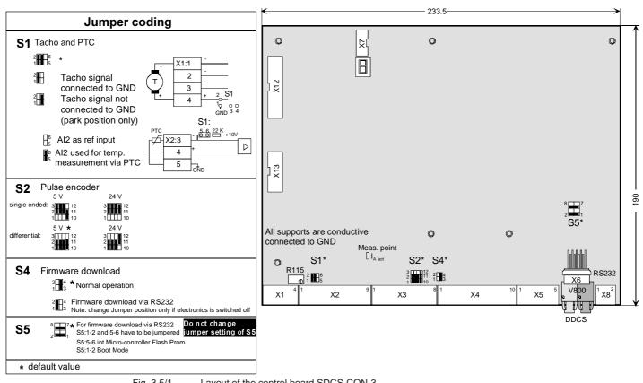
Fig. 3.5/1 Layout of the control board SDCS-CON-3
