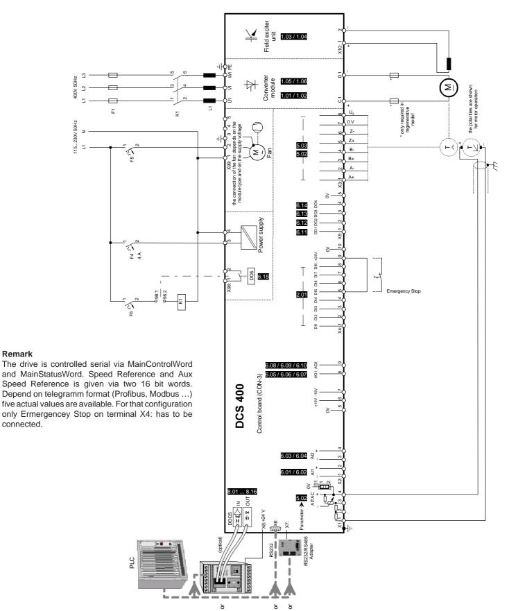
Fig. 5.3/2: Connection example for a serial communication of a PLC
