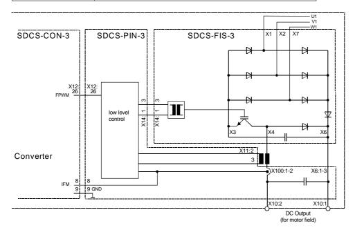
Fig. 3.7/2 Diagram of the field exciter unit
