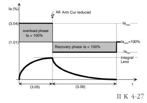
The overload phase is set using parameters Arm Cur Max (3.04) and Overload Time (3.05). The recovery phase is set using parameter Recovery Time (3.06). In order not to overload the Motor, the l<sup>2</sup>t-plane of the two phases have to be identical:
