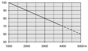
Fig. 2.1/1: Effect of the site elevation above sea level on the power converter's load capacity
