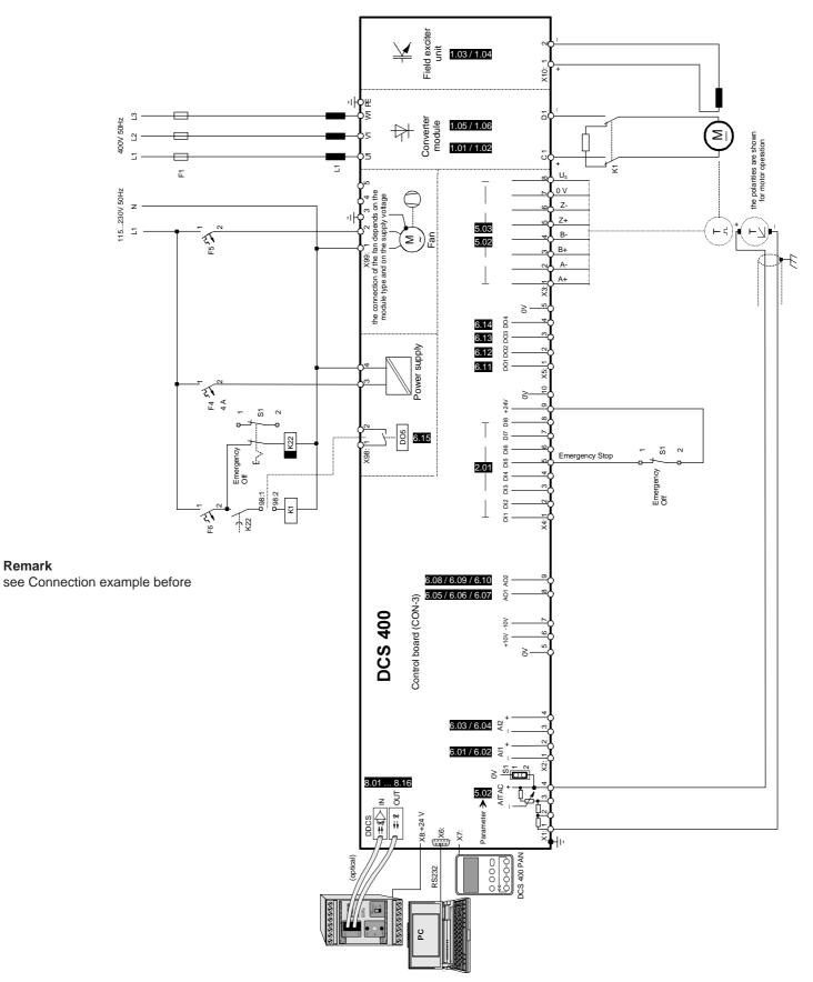
Fig. 5.3/4: Connection example with DC breaker and controlled deceleration
