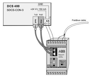
Fig.: 7.3/2 Connection of Fieldbus Adapter to DCS 400
