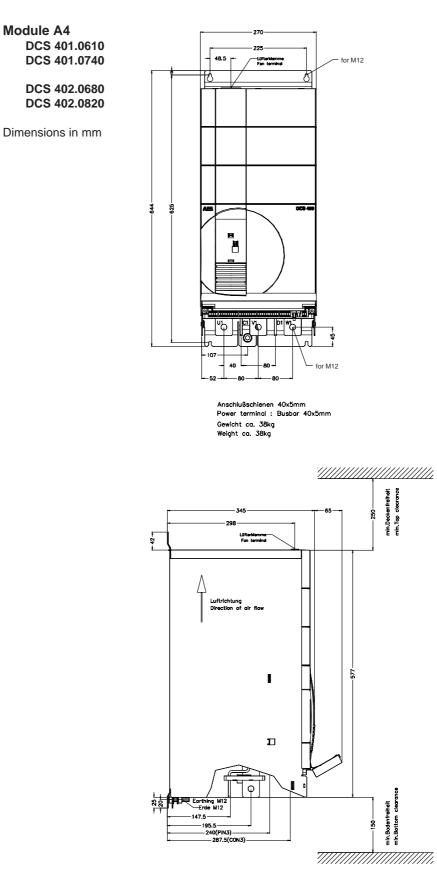
Fig. 3.1/2: Dimension drawing A4-Module
