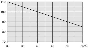
Fig. 2.1/2: Effect of the ambient temperature on the converter module load capacity.
