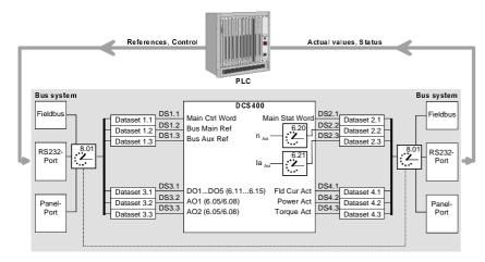
Fig.: 7/1 Data transmission between PLC and DCS 400
