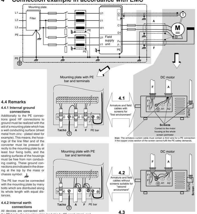
the PE bar by the mounting plate (and also by PE conductors), and the PE bar is earthed via the PE conductor of the 3-phase power cable.
