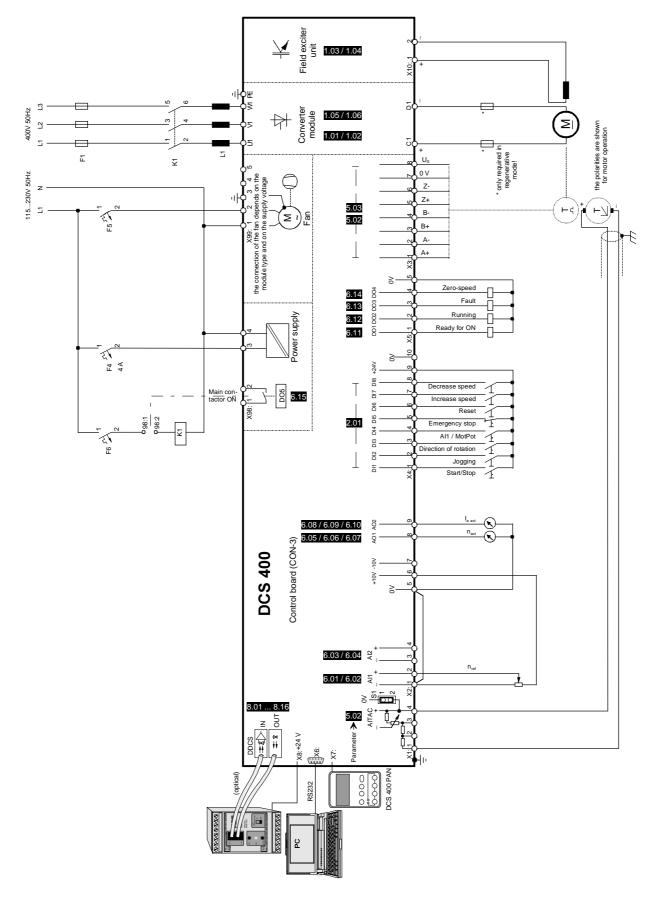
Fig. 4.2/4: Connection example application-Macro 4 - Hand/MotPot
