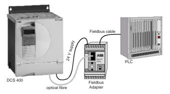
Fig: 7.3/1 Connection of a Fieldbus Adapter to DCS 400 and PLC
