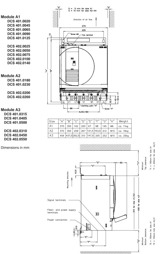
Fig. 3.1/1: Dimension drawing A1, A2, A3-Module
