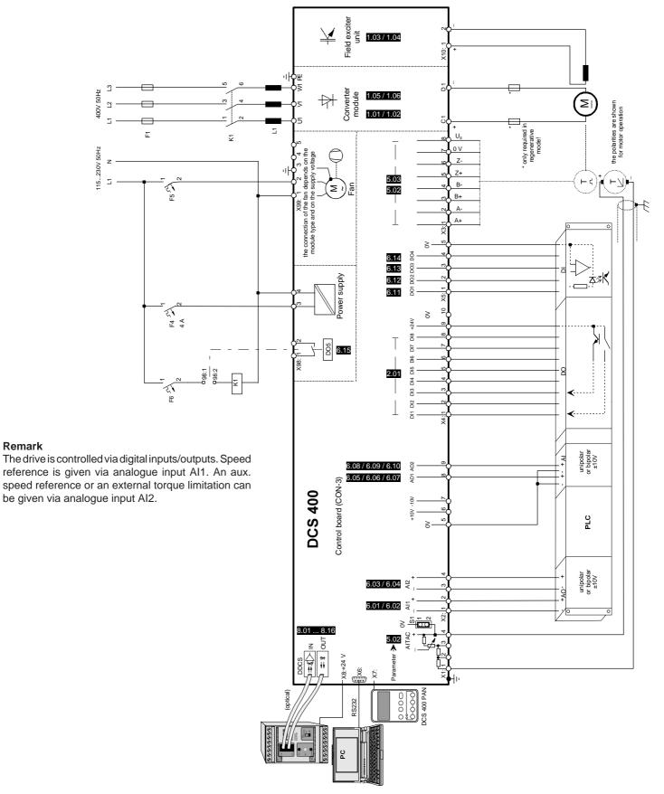
Fig. 5.3/1: Connection example for digital and analogue coupling of a PLC
